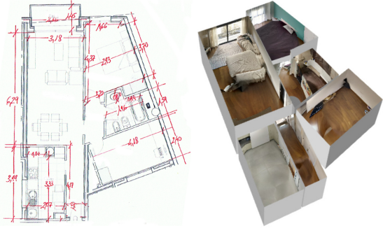
Figure 6: Apartment with 7 rooms (Tab. 1 House2). On the left, the blueprint assumed as ground-truth with its real measures inserted by the designer. On the right, our reconstruction.
