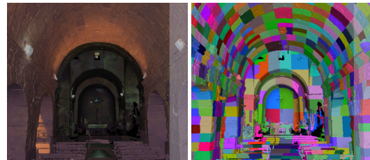
Figure 4: Sant'Antioco Basilica. Patch refinement: 1665 patches with a total of 1.3M samples, rendered at 100 fps on a 1024x768 window, with elliptical splats enabled.
