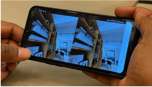
Figure 9: SPIDER-mobile application. The stereoscopies renderer is deployed on Android platform, and the indoor scene can be interactively explored through touch interface or by using IMU sensors for simulating head movements and ready for VR headset like Google Cardboards.
