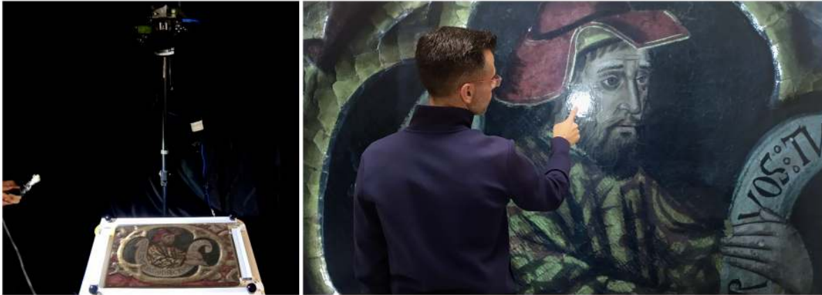
Fig. 1. Capture and relighting of a painting (panel of the polyptych retable of Saint Bernardino (1455), Cagliari, Italy). The optical response of the painting surface to variable illumination is measured by taking a few tens of photos using a fixed reflex camera and a hand-held LED (left). The Multi-Light Image Collection is then transformed to a shape and material representation, which is used for interactive relighting (right)
