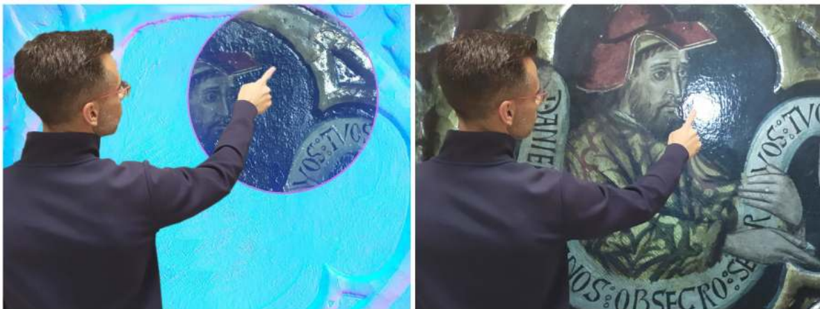
Fig. 25. Exploration of a painting (panel of the polyptych retablo of Saint Bernardino (1455), Cagliari, Italy). The user explores the dataset using visualization lenses and relighting on a large multitouch screen. Left: the outside of the lens shows the normal map, while the inside shows a relighting from SV-BRDF. Right: the user interactively controls a spot light to relight the painting.
