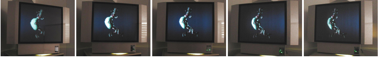
Figure 2. Holographic display example. The images that were taken from different positions in front of the display. The 3D model is an abdominal aortic aneurysm reconstructed from CT data.
