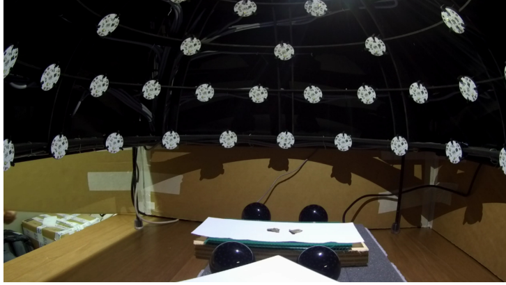
Figure 7. The acquisition setup: the dome is placed in order to have the object near the center of its sphere with its flatter part perpendicular to the camera axis.
