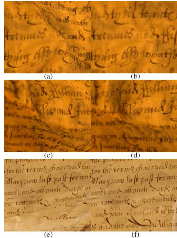
Figure 5: Interactive browsing of damaged documents. Severely damaged documents are acquired in 3D using a Structure-from-Motion approach. A dynamic flattening is performed while the user browses the document in order to increase its readability. We show sections of the mesh rendered in local-affine mode without flattening (left) and with local-flattening mode (right). Note that the original wrinkles remain visible since the shading is baked into the texture. Images courtesy of Pal et al. [PTW13b]
