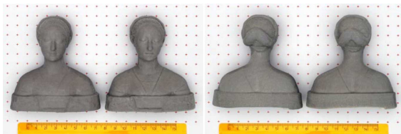
Figure 2: Color enhancement. The color-enhancing technique in action on the Laurana model [Aim03]. Represented objects are less than 10 cm tall (crosshairs are 1 cm spaced). In each pair of images, the left model is a standard uniform color reproduction, while on the right the same 3D model has been printed with enhanced color: many small details whose shading is canceled by the sub-surface scattering effect are again visible in the model on the right. Images courtesy of Cignoni et al. [CGPS08].
