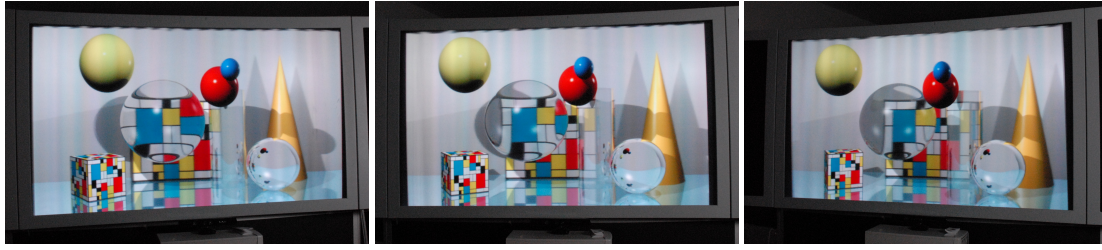
Figure 3: Static scenes rendered in a 35MPixel large scale HPO light field display. Pictures acquired live with a hand held camera. The calibrated system is able to provide correct motion parallax effects and a good registration between displayed object space and physical space.
