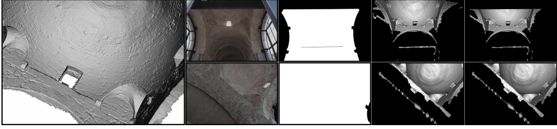
Figure 3: Weighting Function Computation. From left to right: rendered point cloud; photos being blended; user defined stencil masks; per-pixel weights; masked per-pixel weights.
