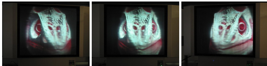
Fig. 1. Real-time interaction with the light field display. Real-time inspection of a large volumetric model containing a CT dataset of a biological specimen. Pictures are taken with a hand-held camera at different viewing angles, in order to highlight the horizontal parallax of the light field display.
