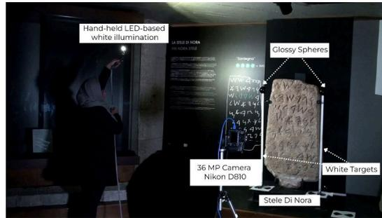
Figure 6.8: **Nora Stone acquisition.** We performed an on-site free-form MLIC acquisition, with a fixed 36.3 Mpixels DSLR FX Nikon D810 Camera with a 50mm AF Nikkor Lens and a moved handheld white LED (5500K) covering the entire visible spectrum with more than 60 images. The acquired data has been calibrated with four glossy spheres (for light direction), and with a white frame positioned around the object
