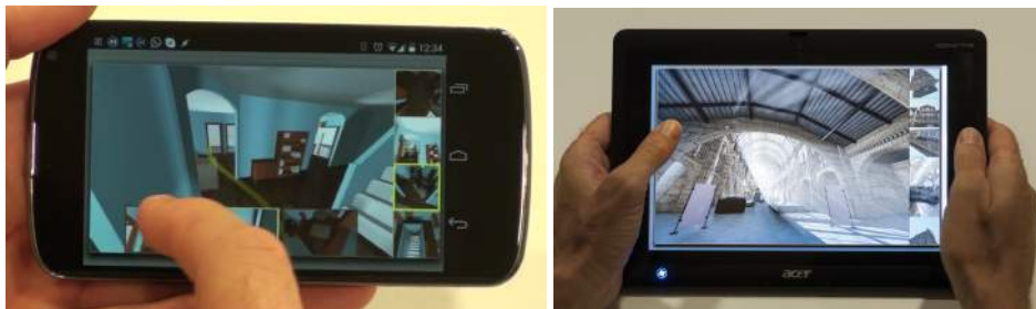
Figure 10.1: Mobile web-based exploration. The graph-based representation is exploited for providing visual indexes for the 3D scene and for supporting, even on low-powered mobile devices, interactive photo-realistic exploration based on precomputed imagery. On the left, browsing the German Cottage model on a Nexus 4 phone; on the right browsing the National Museum model on an Acer Iconia tablet.
