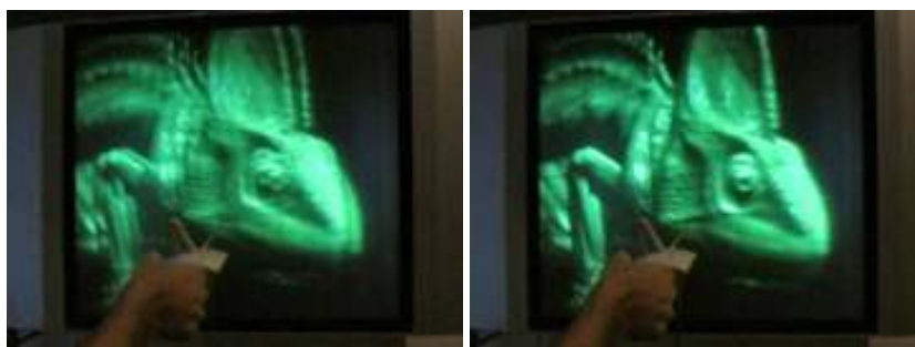
Figure 5.6: Dynamic tile misalignment effect. The 96 display projectors are updated in batches of 16 projectors each, which can lead to artifacts in dynamic motion if the rendering rate is too slow (left). These artifacts disappear when the image is static (right).
