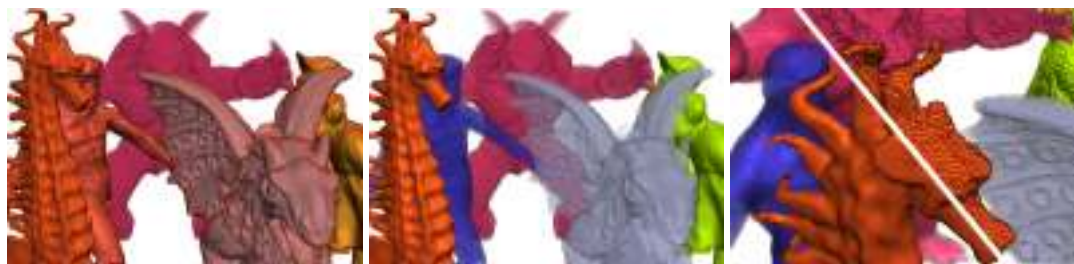
Figure 4.1: Rendering of a labeled scene. Left: The usual linear interpolation method suffers from color bleeding, since interpolated values generate false colors when accessing transfer functions even when using pre-integration. Middle: using split-voxels, all segmented models keep their color. Right: a close-up of the scene with low pixel tolerance shows how the split-voxel method preserves boundaries even at very low levels of details, instead the nearest method suffers from low quality edge representation.
