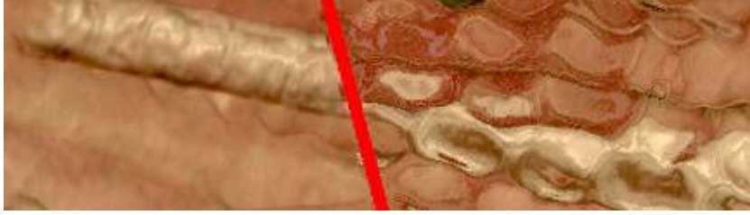
Figure 3.5: Detail comparison showing the refraction effect. With refraction enabled (right), ray direction is changed at each integration step according to Snell’s law, and fine details in transparent objects become visible. The view-dependent effect is evident when seen on the light-field display.
