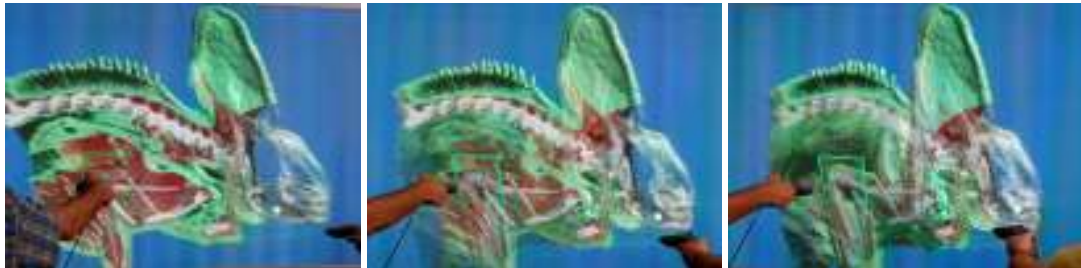
Figure 1.1: Multi-user interactive exploration of a chameleon 1-GVoxel dataset on a 35-MPixel light-field display. Users freely mix and match 3D tools creating view-dependent illustrative visualizations. Objects appear floating in the display workspace, providing correct parallax cues while delivering direction-dependent information.
