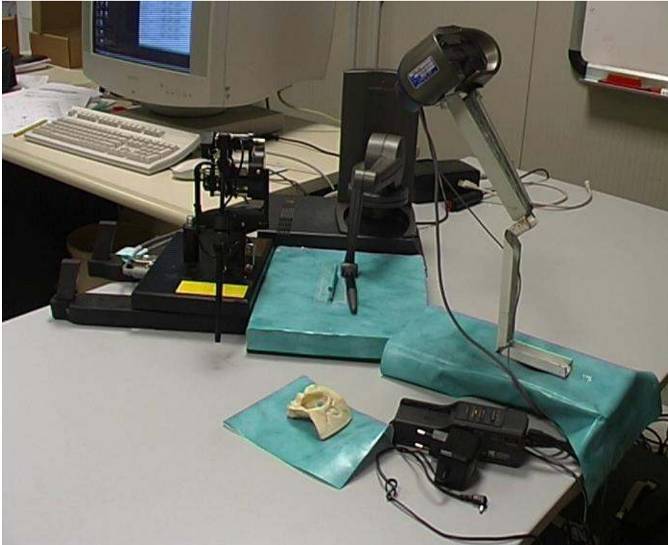
Figure 11.3.: The current Ierapsi surgical simulator set-up. Note the Phantom Desktop haptic device for the dominant hand; the Phantom 1.0 haptic device for the non-dominant hand and the n-vision VB30 binocular display.
