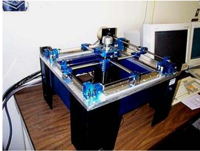
Figure 5.11.: Linear Haptic Display - Excalibur: is a 3 degree-of-freedom haptic device, built for maximum workspace, force output, and structural stiffness. Photo taken from University of Washington web resource http://brl.ee.washington.edu .
