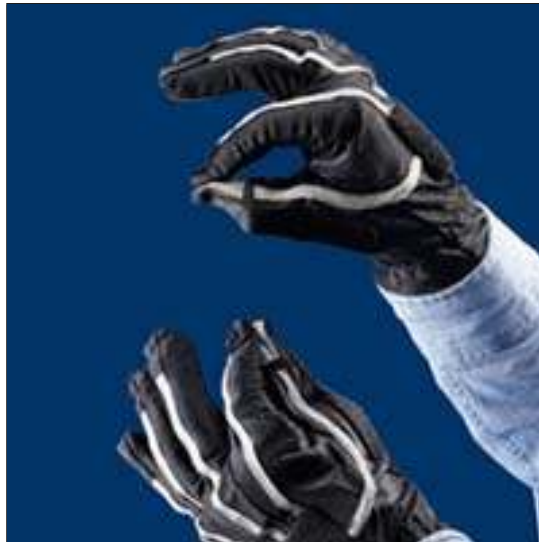
Figure 5.4.: PINCH Glove : The PINCH System uses cloth gloves with electrical sensors in each fingertip.
