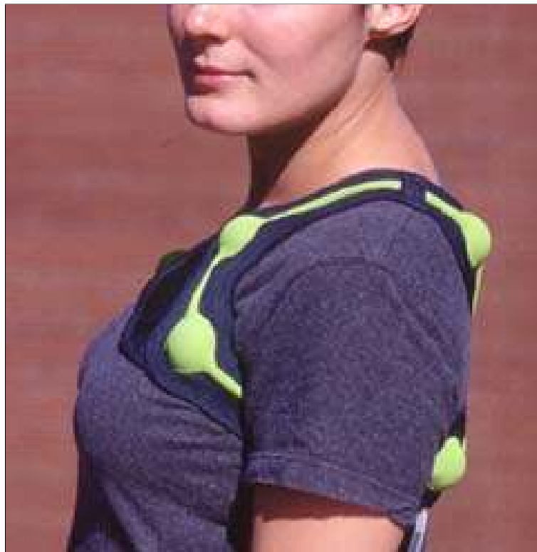
Figure 5.8.: Tactile vest: a wearable device that provides haptic feedback to the torso, based on Nitinol, a shape memory alloy (SMA). Photo taken from Berkeley University site http://kingkong.me.berkeley.edu .
