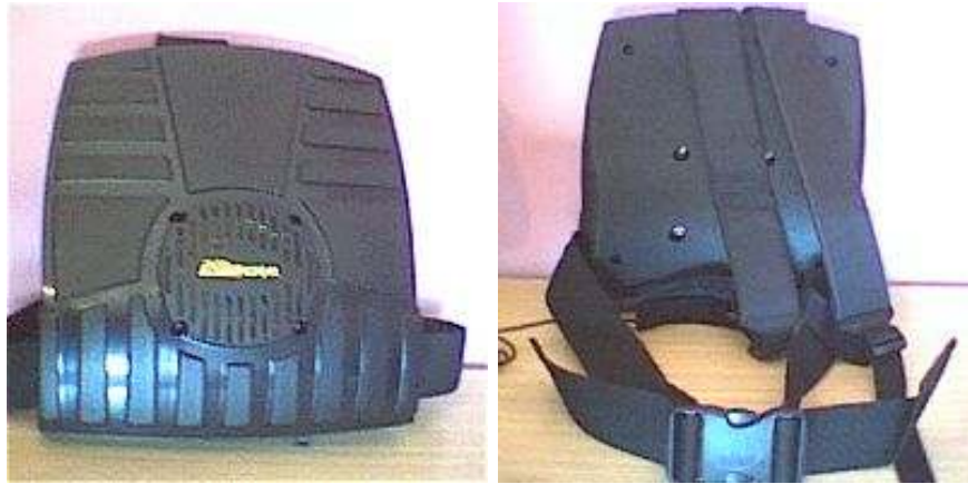
Figure 5.7.: Aura Interactor: it creates body-pulsing vibrations keyed to the on-screen action. Photo taken from Aura systems site.
