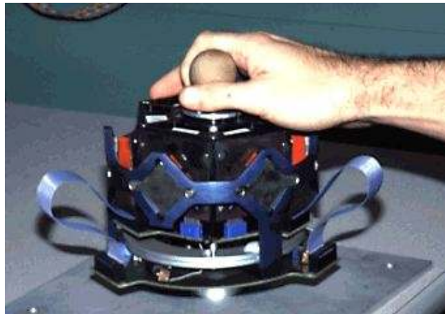
Figure 5.12.: CMU Magnetic Levitation Haptic Interface: the magnetic levitation technology uses Lorentz forces to stably levitate and control a rigid body. Photo taken from Carnegie Mellon University site http://www-2.cs.cmu.edu/msl/ .
