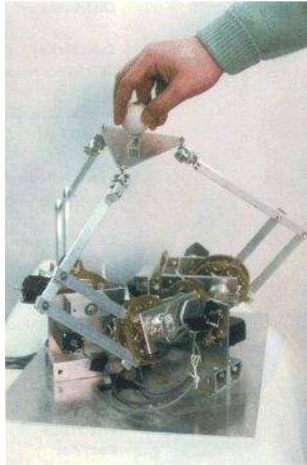
Figure 5.13.: University of Tsukuba Haptic Master: Haptic master system employs three sets of parallelogram linkages (pantographs) instead of linear actuators. Photo from web resource http://intron.kz.tsukuba.ac.jp .
