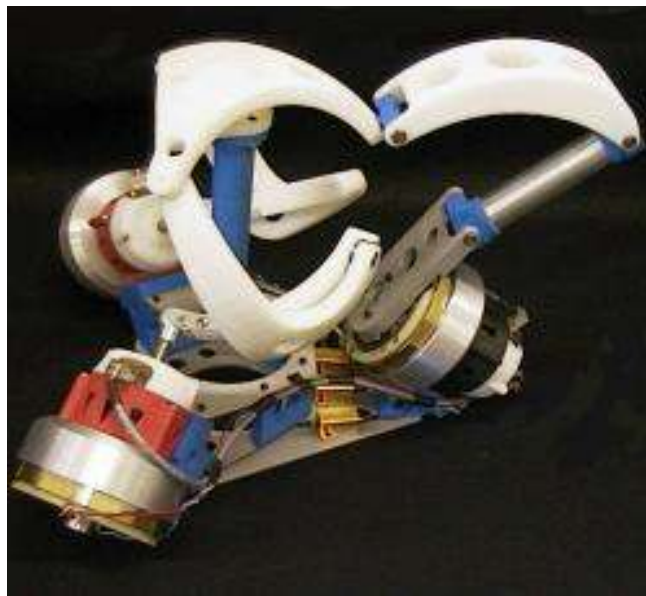
Figure 5.15.: SHade : Spherical Haptic DEvice. Photo from University of Laval site http://www.robot.gmc.ulaval.ca/ .
