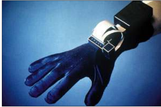
Figure 5.3.: 5DT 5th Glove : The 5th Glove uses 5 fiber-optic flex sensors to generate finger-bend data for 5 fingers. It has an integrated pitch and roll sensor. Photo from Fifth Dimension Technologies site http://www.5dt.com .
