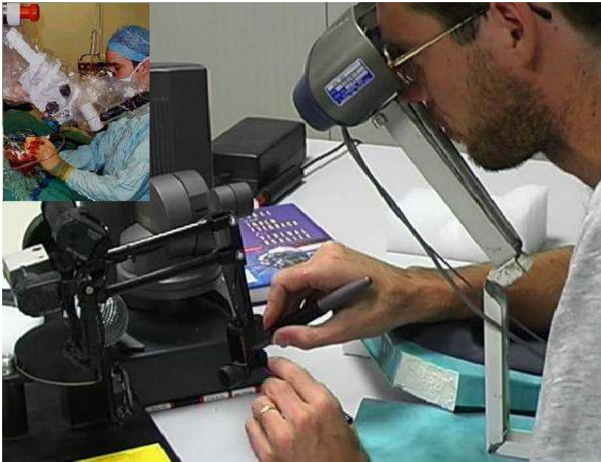
Figure 12.1.: Virtual vs real mastoidectomy surgical setup. The surgeon looks at the region interested by the procedure via a stereoscopic microscope and holds in his hands a high speed burr and a sucker. The main photo shows the virtual simulator setup, while the inset photo represents a typical mastoidectomy surgical theater. Inset photo courtesy of Prof. Bob Stone, Virtual Presence Ltd.
