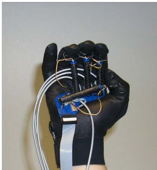
Figure 5.5.: Rutgers Masters II : RM-II reads hand gestures (hand-master) and displays forces (haptic-display) to four finger in real time. Photo from Rutgers University site http://www.caip.rutgers.edu .
