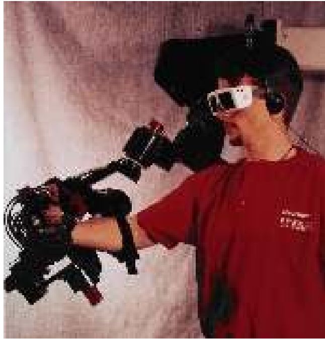
Figure 5.14.: Sarcos Dextrous Arm Master : this device utilizes high-performance hydraulic actuators to provide a wide dynamic range of force extension at relatively high bandwidth on a joint-by-joint basis for 10-DOF. Photo from Sarcos site http://www.sarcos.com .
