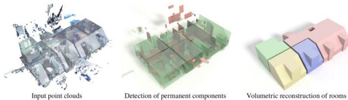
Mura et al. **Piecewise-planar Reconstruction of Multi-room Interiors with Arbitrary Wall Arrangements.**
