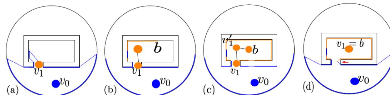
Coverage optimization, by moving to the barycenter of seen geometry
