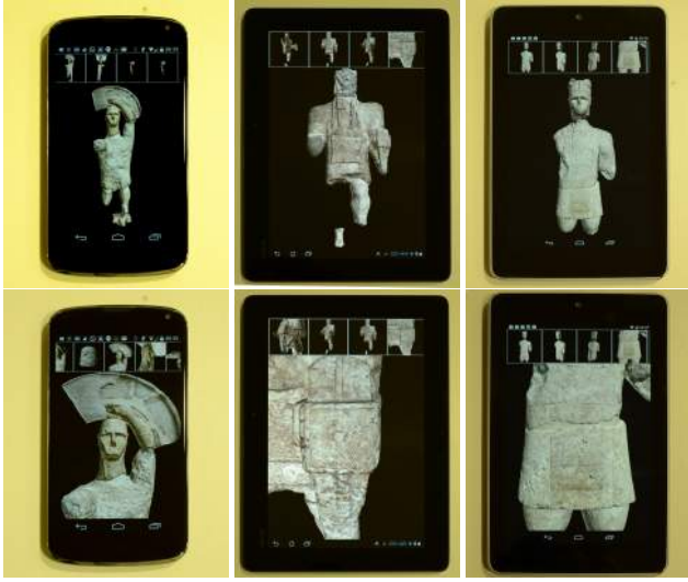
Figure 8: Various levels of detail of a statue. Images correspond to Nexus 4, Asus TF201 and Nexus 7, respectively. Top: View of the whole statue. Bottom: A close-up of the statue showing small-scale details.
