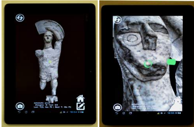
Figure 9: User study performed on a Nexus 7 tablet. ACeViT compared to Virtual TrackBall with fixed pivot and with manual pivot positioning. Left: test scene composed of a detailed surface model composed of 70Mtri. Right: tasks consisted of reaching and shooting specific positions and orientations indicated by green cylinders.
