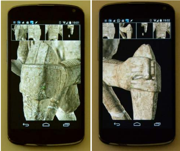
Figure 4: Detail of model interactively rendered on a Nexus 4 smartphone. This 70Mtriangles model is colored using post-restoration color data. Note how our compression preserves extremely high quality details in shape, normal, and colors.
