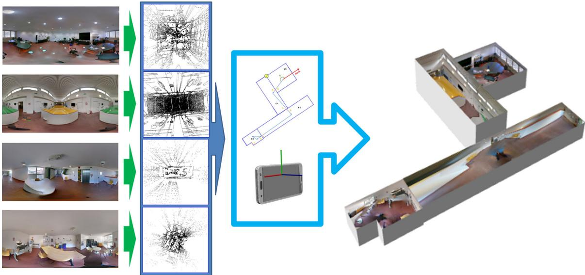
**Figure 3:** We take as input one omnidirectional image for each room and project the image gradient map to a plane to highlight and extract the room shape. We iterate the method to map and reconstruct the entire floor plan, using the IMU to recover scale and relative position of rooms. As a result, we obtain a 3D representation of the captured environment, along with its visual representation through spheremaps.
