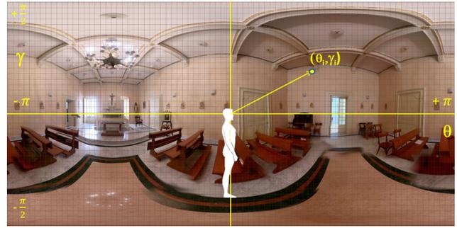
**Figure 2:** The equirectangular image represent all possible views for an observer ideally located in the center of the spheremap, identified by the angles  $\theta$  and  $\gamma$ .
