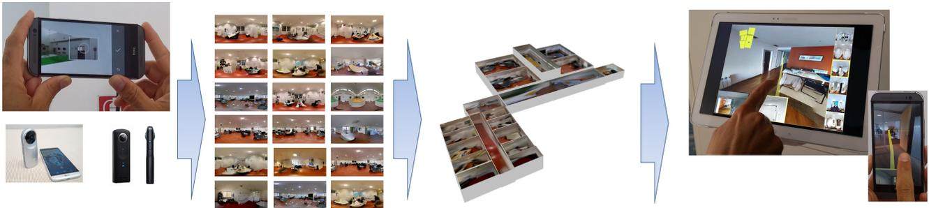
**Figure 1:** Starting from panorama images generated with the aid of commodity mobile devices, our methods rapidly compute visual and structural 3D models of indoor environments scaled to their metric dimensions. The resulting 3D floor plans of multi-room environments can be used for a variety of planning applications, while the visual models provide location awareness within mobile application specifically developed for touch interaction on smartphones and tablets.
