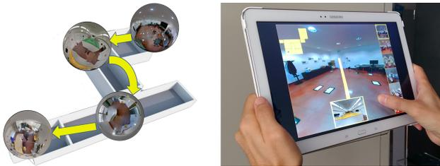
**Figure 5:** Each node of the exploration graph is represented by a spheremap/room, whereas the edges (yellow) are the transition between adjacent rooms, which are generated by view interpolation using the reconstructed structural geometry. The resulting model can be quickly explored visually on a mobile platform even in presence of low-bandwidth networks.
