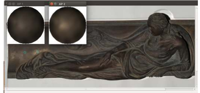
Figure 8: The RTI analysis interface allows the display of a reflectance image related to single point or ROI, allowing an easy comparison of different material properties.
