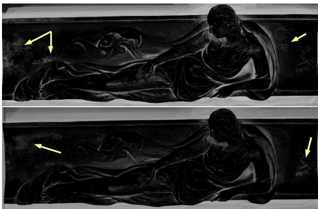
Figure 12: Top: OD map estimated on Visible RTI stack for the statue. Bottom: OD map estimated on IR RTI stack for the statue. While body contours are well shown due to the detection of shadow, in the region indicated with arrows, higher values show differences in local material reflectance due to different/missing patination.
