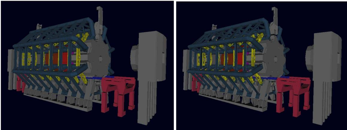
Figure 1: A view of the whole ATLAS Experiment Pit. Comparison between full (left, 1,072,858 triangles) and adaptive resolution (right, 41,487 triangles).
