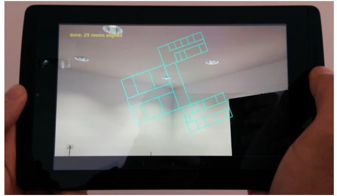
Fig. 6. **Indoor capturing.** The system to capture building interiors and automatically generate floor plans scaled to their metric dimensions.
