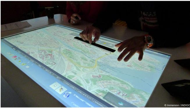
Fig. 4. **INDIGO Tangible Ruler.** Users are able to measure digital maps with a tangible ruler. The digital scale around the objects automatically adapts to the maps scale.
