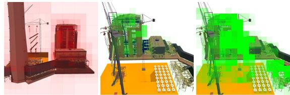
**Figure 4:** Left: Visualization of the occlusion-query overdraw for primary rays, where reddish regions have high overdraw. Middle and right: Illustration of the reduced spatial coherence using diffuse rays with length 10 and 1000, respectively. An opaque green screen-space tile means that its rays potentially intersect  $> 2M$  triangles.
