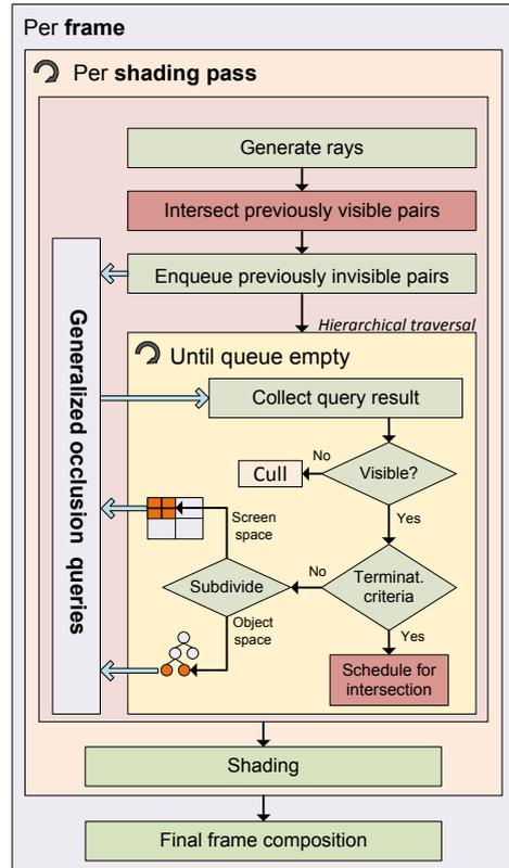
Figure 2: Overview of the proposed algorithm, CHC+RT.
