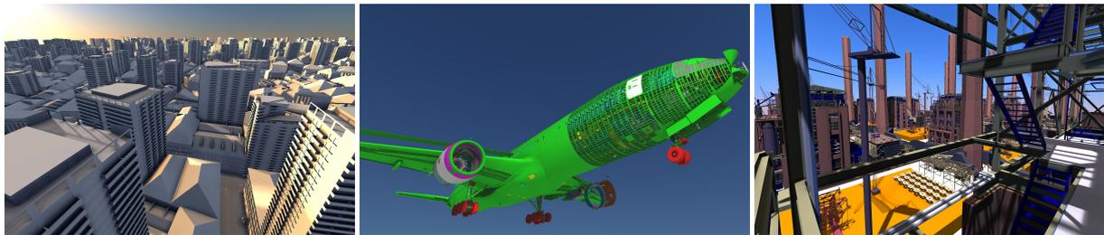
**Figure 1:** Sample images from our interactive OpenGL ray tracer using the CHC+RT algorithm. From left to right: A City model with 138M triangles (7.89GB), the Boeing 777 model with 350M triangles (18.9GB) and 16 copies of the Powerplant model with 205M triangles (11.4GB). Our algorithm based on hierarchical occlusion culling allows a simple scheduling scheme for managing out-of-core scenes and also significantly accelerates OpenGL-based ray tracing in complex scenes.
