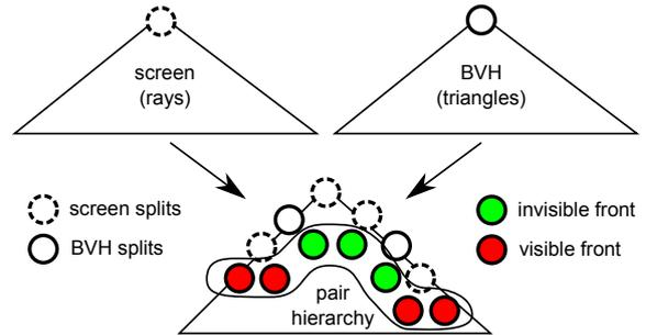
**Figure 3:** Illustration of the query-pair hierarchy. The interior nodes of the hierarchy correspond to either screen-space splits or object-space splits. The leaf nodes belong to either the visible front (rays and triangles that can intersect) or the invisible front (rays and triangles that cannot intersect).
