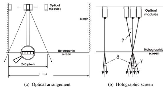
Figure 1: **Optical arrangement.** The light beams are generated through a modular light modulation system arranged in a specific geometry and the holographic screen makes the necessary optical transformation to compose these beams into a continuous 3D view.
