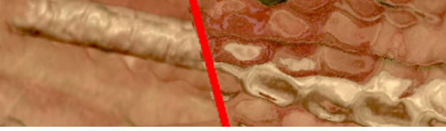
Fig. 4 Continuous refraction. With refraction enabled (right), ray direction is changed at each integration step according to Snell’s law, and fine details in transparent objects become visible. The view-dependent effect is evident when seen on the light field display.
