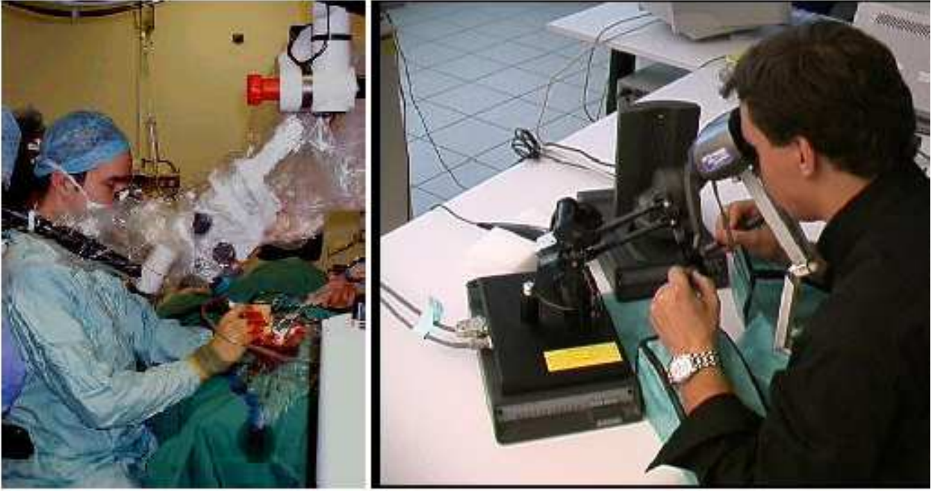
Figure 1: Surgical equipment and Simulator setup: Left: Real surgical environment, the surgeon keeps in his hands a high-speed rotating burr and a sucker and looks through a microscope. Right: The CRS4 simulator provides both haptic and binocular feedback.
